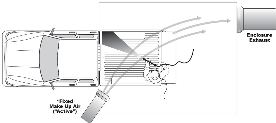
\* The volume of air supplied by this unit is dependent on the size of the enclosure exhaust unit, therefore the volume of make up air is determined on a case by case basis.
